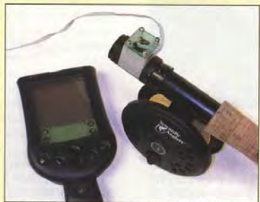
The Casting Analyzer was developed at the University of Michigan by co-author Noel Perkins. It detects rod speed and records the information on a hand-held computer.
