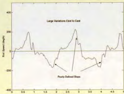
Figure 3a. Beginning casters display large variations in rod speed and poorly defined stops.
