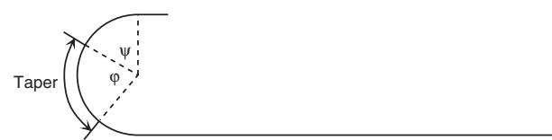
Figure 6 Three generic positions of the taper. (a) Taper wholly within traveling line, (b) taper partly within traveling line, (c) taper wholly within loop.
