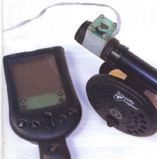
Noel uses a Palm hand-held computer to monitor his casting action with a micro-electromechanical sensor linked up to the butt of the rod.
